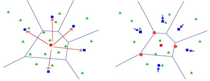
Figure 5. Schematic of load balancing. (Left) The center matcher requests help from its neighbors. Triangles are the subscriptions centers of clients. (Right) Neighbor matchers move their sites closer to make the center region smaller. Note that some subscription centers are now in neighbor regions, the ownerships thus are transferred (e.g., the circles at the boundaries).
